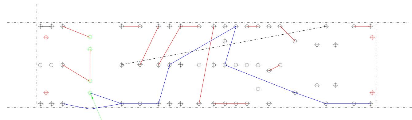
Black drill marks are for turrets. Red drill marks are for mounting holes. Green drill marks are for snap-in capacitor terminals. Note that grid resistors for V1a are not on the turret board: they connect directly to the tube socket. The four grid resistors for the power tubes are also on the tube sockets. One lead from the standby switch goes to the center tap (red) of the output transformer.
