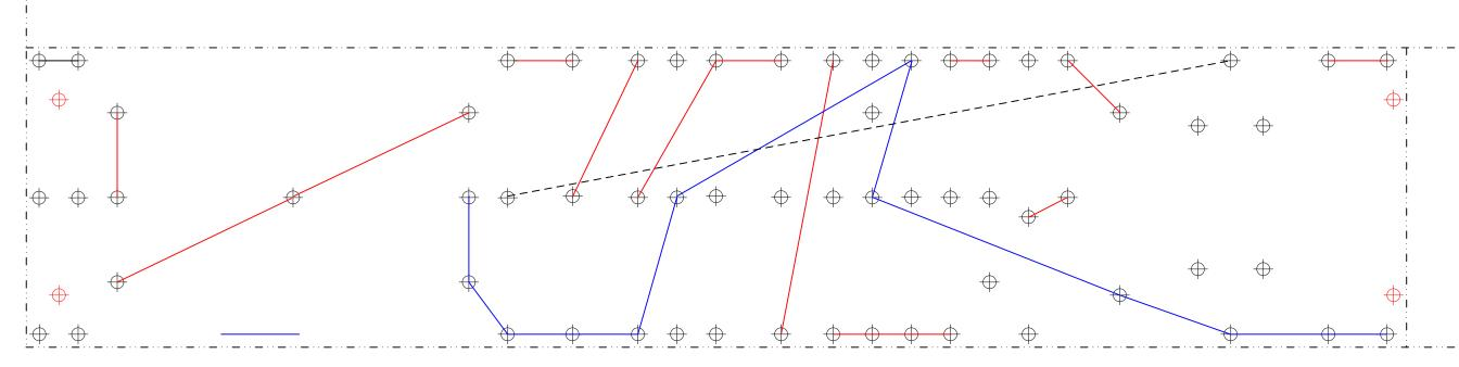
Black drill marks are for turrets. Red drill marks are for mounting holes. Green drill marks are for snap-in capacitor terminals. Note that grid resistors for V1a are not on the turret board: they connect directly to the tube socket. The four grid resistors for the power tubes are also on the tube sockets. One lead from the standby switch goes to the center tap (red) of the output transformer.
