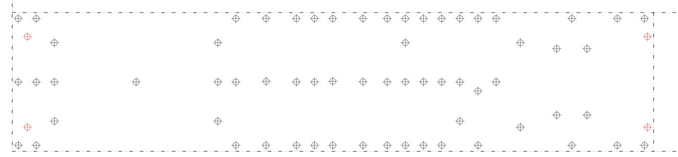
Black drill marks are for turrets. Red drill marks are for mounting holes. Green drill marks are for snap-in capacitor terminals. Note that grid resistors for V1a are not on the turret board: they connect directly to the tube socket. The four grid resistors for the power tubes are also on the tube sockets. One lead from the standby switch goes to the center tap (red) of the output transformer.
