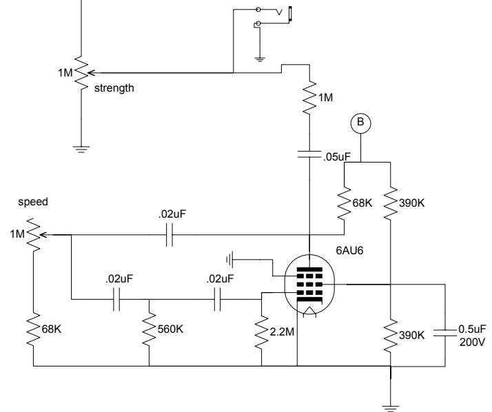
All capacitors 600V unless otherwise noted, all pots audio taper, pots coded 137741 (CTS made 1957, 41<sup>st</sup> month), speaker 285732 (Rola 1957, 32<sup>nd</sup> month). Number on amp 1127, probably means built November, 1957. Measured voltages are in red.
